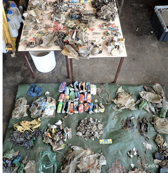
Figure 22: Characterisation of waste in stormwater discharge (Cedre)
